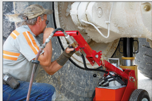
The High Tonnage Jumbo Jack in use.
